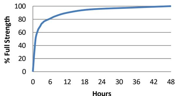
Graph shows typical strength development of bonded components at 23°C. Curing at higher or lower temperatures may affect cure speed.
