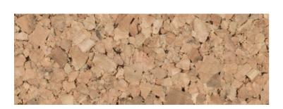
**ETP021** is a polyurethane cork agglomerated material with low density and high compressibility, together with high thermal insulation.
